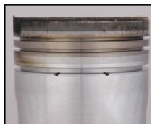
* Ring-zone condition after 8,824 hours and up to 3,052 hours drain interval.
